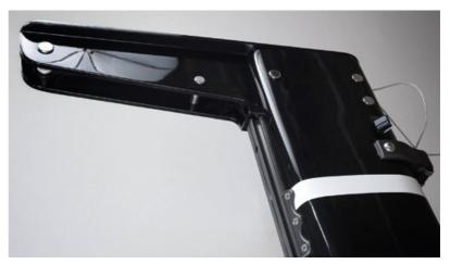
The carbon masthead eliminates the danger of galvanic corrosion and cuts back on weight while the anodized aluminium or acetal low-friction sheaves allow easy hoisting of the sails. The anodized aluminium halyard fairlead then prevents the spinnaker halyard from chafing against the mast.
